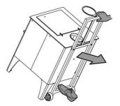
Your ESSE Garden Stove comes supplied with the wheel trolley in position. To move the appliance, place one foot on the base of the trolley, and gently rock backwards, onto the two wheels. You can now carefully pull your ESSE Garden Stove into position.
