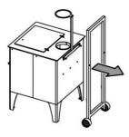
Once in position, the trolley can either be removed if desired, or left attached. To remove the trolley, use a 10mm spanner to remove the two retaining nuts. Remove the trolley, before replacing the two retaining nuts.
